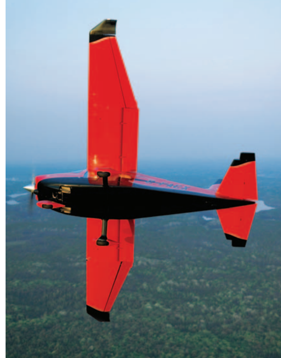
The tapered wing reduces drag, while delivering better lift and STOL capability.
