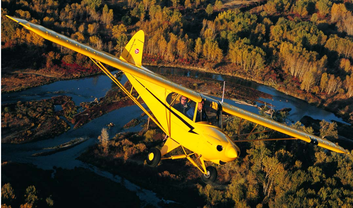
Above: Responsive controls and low fuel burn at typical speeds of 90 to 110 mph as well as good visibility make the SPORT CUB fun to fly. Below: Standard vortex generators improve controllability, especially at low speeds of 50 to 60 mph typical on approach to short strips. Opposite: The prototype airplane we flew, N502CR, was equipped with optional 8.00 x 6 tires and a McCauley metal propeller.
